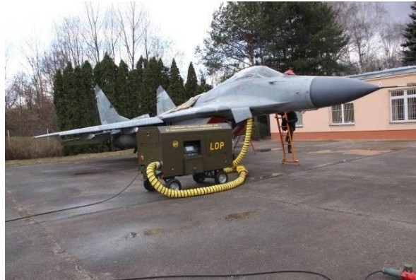
Fig. 6. Aircraft Air Dehumidifier Source: [LOP WCBKT].
